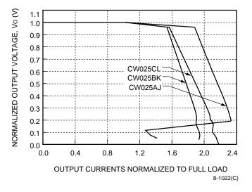
Figure 2. CW025 Dual Output-Series Normalized Output Current vs. Normalized Output Voltage at V<sub>I</sub> = 48 V and T<sub>C</sub> = 25 °C
