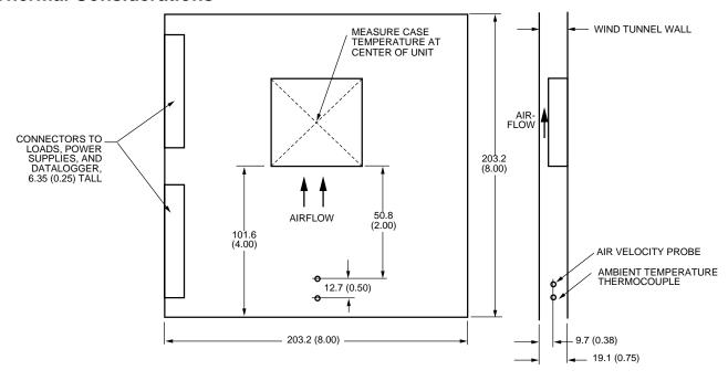
Note: Dimensions are in millimeters and (inches). Drawing is not to scale.
