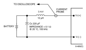
Note: Input reflected-ripple current is measured with a simulated source impedance (LTEST) of 12 µH. Capacitor Cs offsets possible battery impedance. Current is measured at the input of the module.
