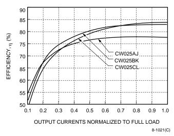
Figure 3. CW025 Dual Output-Series Efficiency vs.
