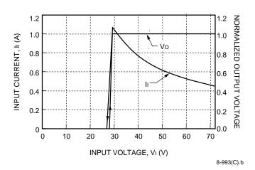
Figure 1. CW025 Dual Output-Series Input Current and Normalized Output Voltage vs. Input Voltage at Full Load and Tc = 25 °C
