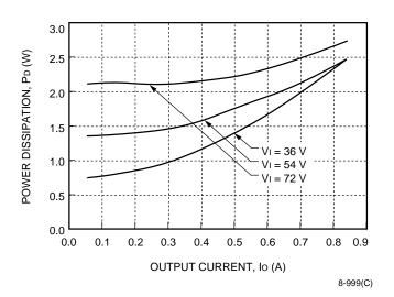
Figure 18. 15 V Output Power Dissipation vs.
