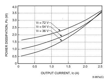
Figure 16. 5 V Output Power Dissipation vs. Output Current
