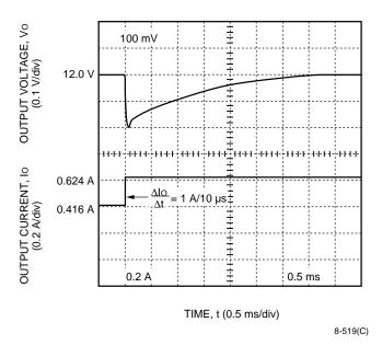
Figure 8. CW025 Dual Output-Series Typical 12 V
