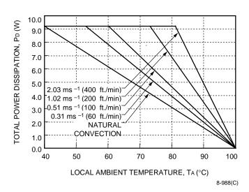
Figure 19. Total Power Dissipation vs. Local
