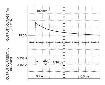
Figure 6. CW025 Dual Output-Series Typical 15 V Output Voltage Response to a Step Load Change from 50% to 25% of Io, max at VI = VI, nom and Tc = 25 °C
