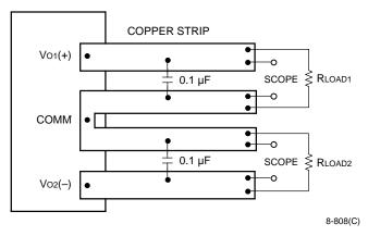
Note: Use a 0.1 µF ceramic capacitor. Scope measurement should be made using a BNC socket. Position the load between 50 mm (2 in.) and 75 mm (3 in.) from the module.
