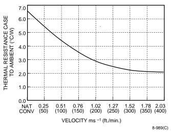
Figure 20. Case-to-Ambient Thermal Resistance vs.
