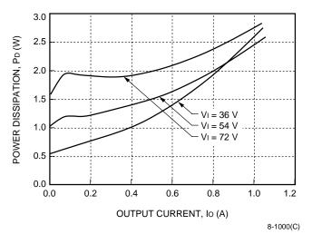
Figure 17. 12 V Output Power Dissipation vs.
